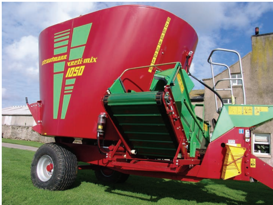
The Strautmann C-conveyor can be used as a standard crossover conveyor, as a movable crossover conveyor and as an "elevating conveyor".
