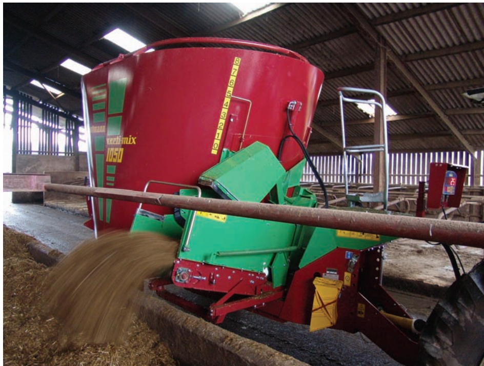
The Strautmann C-conveyor permits discharge heights of 1.40 m.
